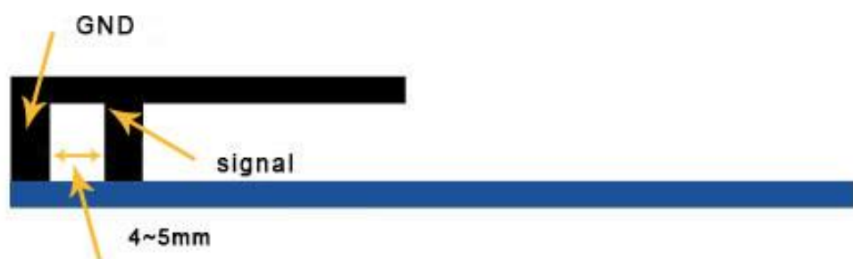
Figure 13. Location of signal point and GND point for PIFA antenna
